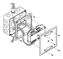
**SIGA-MCC1S:** mount the UIOxR motherboard inside a suitable EDWARDS enclosure with screws and washers provided. Plug the module into any available position on the motherboard and secure the module to the motherboard with the captive screws. Wiring connections are made to the terminals on the motherboard (see wiring diagram). UIOxR motherboard terminals are suited for #12 to #18 AWG (2.5 mm² to 0.75 mm²) wire size.
